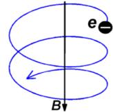
Cyclotron Radiation Emission Spectroscopy (CRES)
