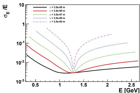
Figure 4: Fractional energy resolution as a function of energy for various beam emittances.
