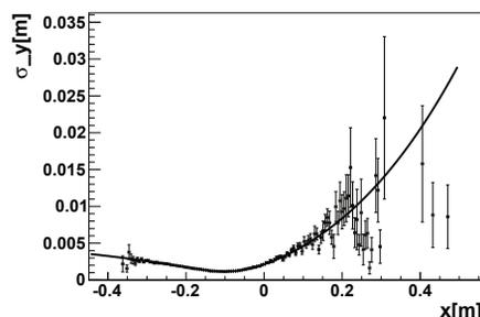
Figure 5: Fit of a simulated electron beam to the *beam size function*.
