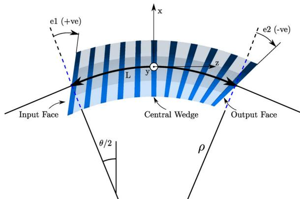
Figure 3: Dipoles in BDSIM are constructed of many small straight sections. Here, the gradual variation from one pole face angle to another is shown.
