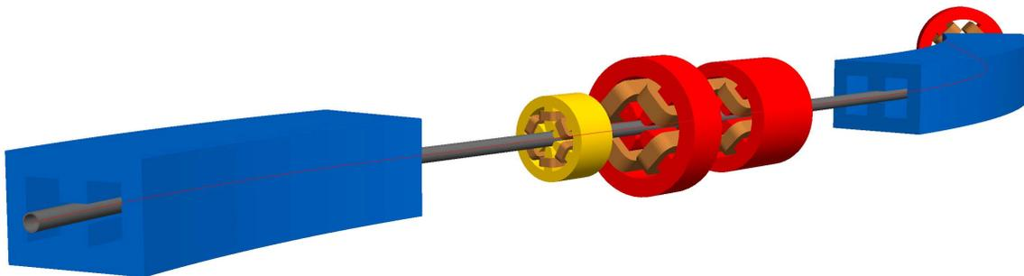
Figure 1: An example beam line built by BDSIM using the *polescircular* geometry style with a single particle passing through (red line).
