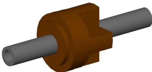
Figure 2: Cavity beam position monitor provided by external geometry in a GDML file in a small example beam line with two drift pieces before and afterwards.
