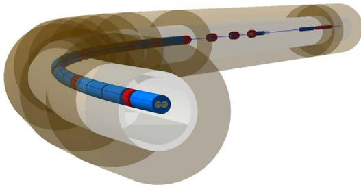
Figure 4: A small section of the Large Hadron Collider modelled in BDSIM showing the capability of producing tunnel geometry that follows the beam line.
