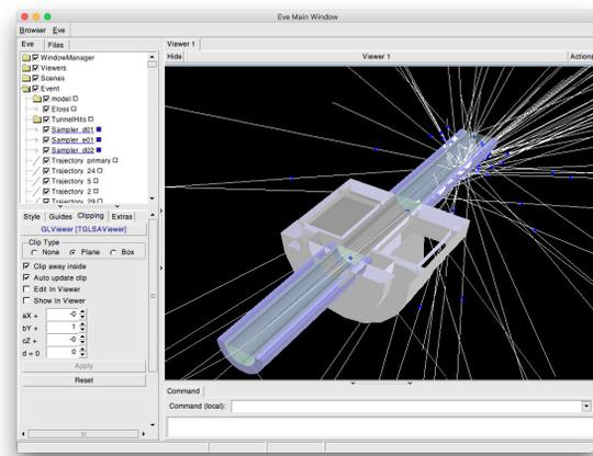
Figure 5: Example event display showing a small lattice in BDSIM that has been exported to a GDML file. The geometry is cut away and the event trajectories are overlaid in the display.
