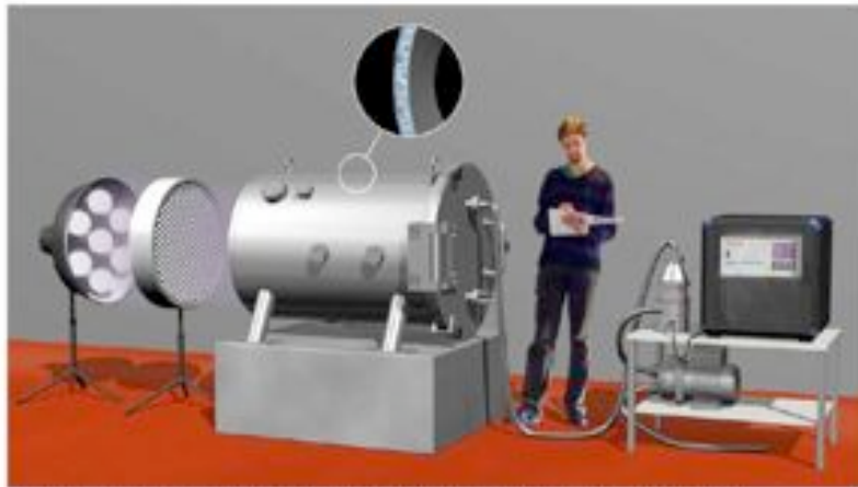
Fig. 2: An impression of SKY-II – a double-skinned chamber with an internal baffle matrix
