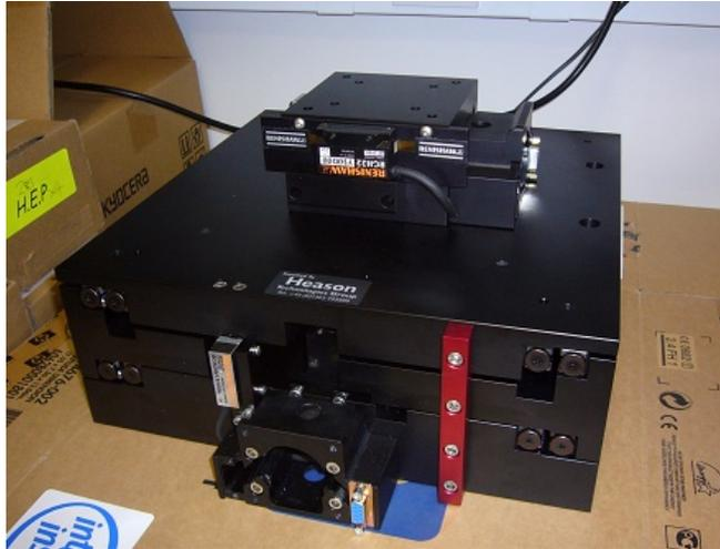
has a **pitch of 2 mm**. Both stages are operated by Baldor DSM hybrid stepper motors. These have an integrated stepper drive equipped with a micro-stepper of up to 51200 steps per revolution. Without micro stepping the motors have nominally **200 steps per revolution**.
