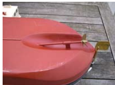
ABOVE: Shows the propeller shaft and skeg in place on the finished model and the rudder mounting
