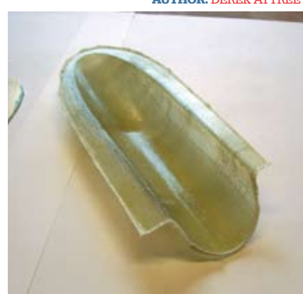
Tunnel removed from the mould
