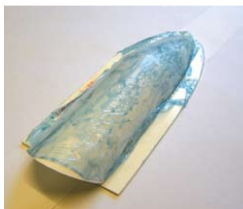
Mould showing release agent (the blue plastic film stuff) after removal of tunnel lay up
