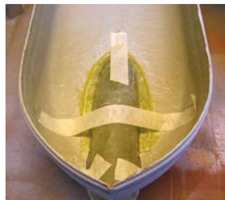
Tunnel taped in place for gluing
