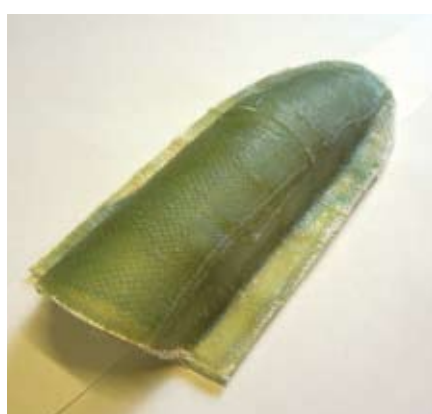
Tunnel moulding in progress
