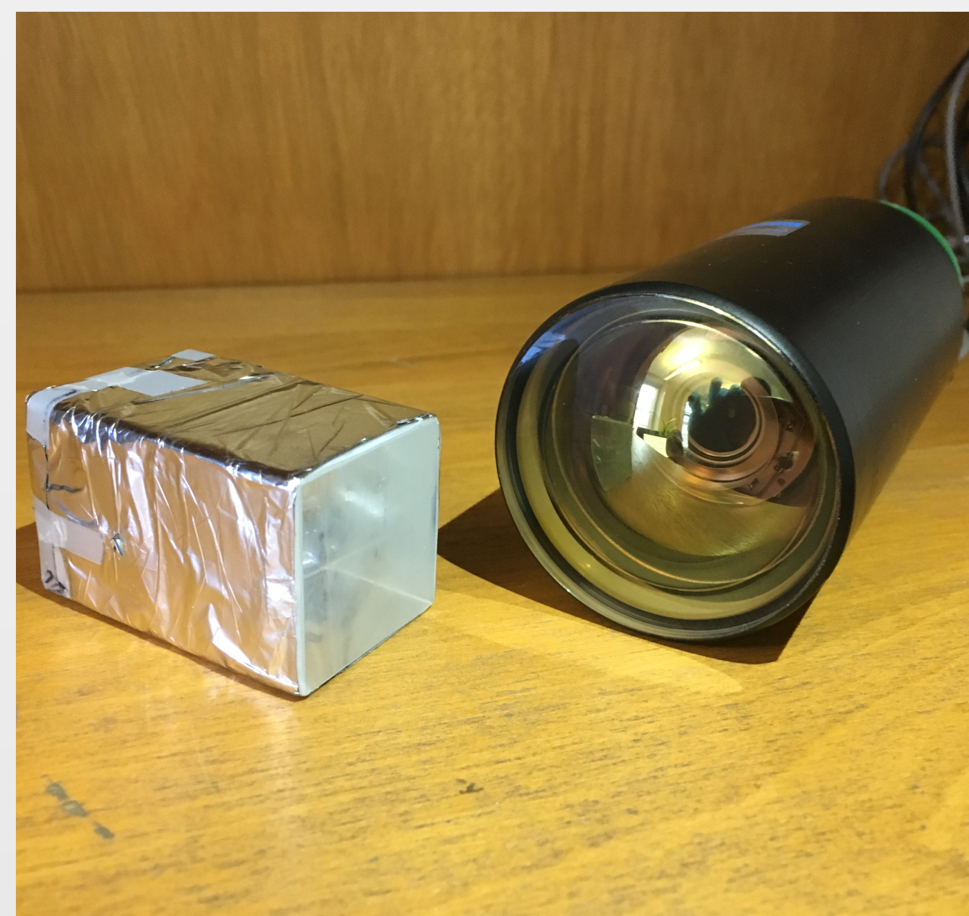
Fig 2. Calorimeter: 3 × 3 × 5 cm module, wrapped in mylar foil and Hamamatsu R13089 PMT.
