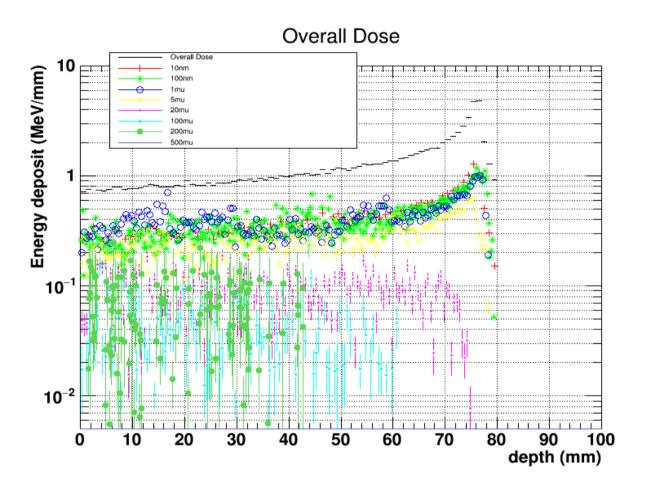
This is because there is a "safety threshold" for ionisation in Geant4: E\_th = 990 eV Geant4 might not accurately simulate energies below that threshold
