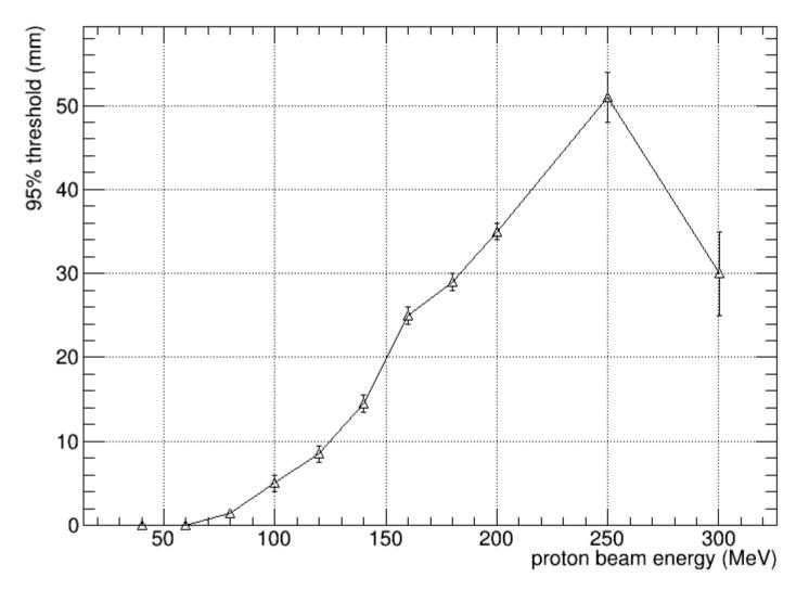
"where dose reaches 95% of predicted dose" Predicted dose: define as the y-axis intersection of the fitted Bragg curve
