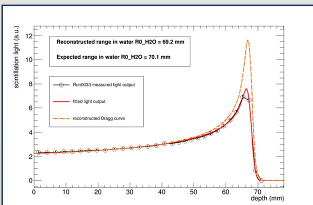
Figure 4: Fit of a quenched Bragg curve to the integrated light output and reconstruction of a pristine Bragg curve.
