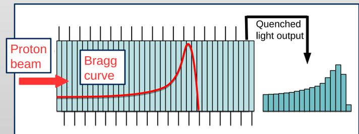
Figure 1: Principle of a range telescope.
