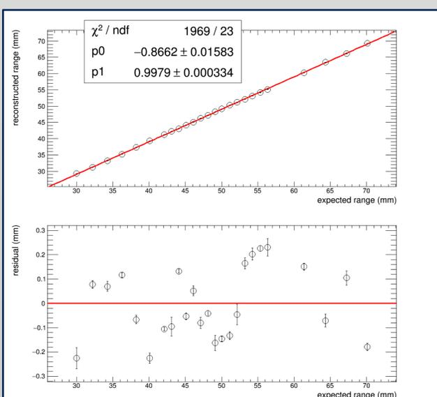
Figure 5: Reconstructed vs. expected ranges and residuals.
