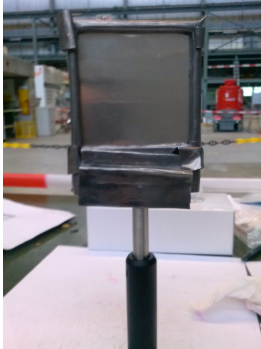
Figure 4.5: A photograph of the aluminium target in its holder with lead shielding covering the plastic holder.
