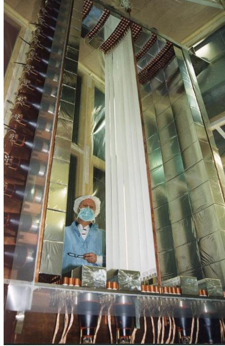
**Figure 4.11.:** *One of the NEMO-3 sectors. The seven strips constituting the source foil can be seen as well as the copper frame they were installed on.*
