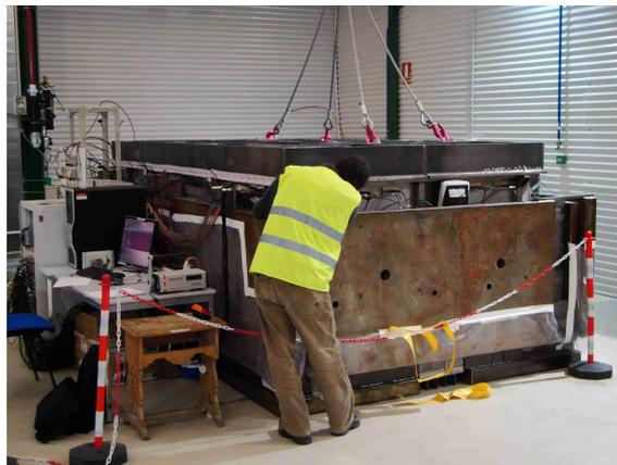
**Figure 7.15.:** *Shielding of the BiPo-3 detector with iron plates outside the stainless steel tank. Lead bricks are placed inside the tank and on top of it.*
