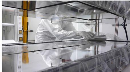
**Figure 7.37.:** *Aluminium calibration foil in a BiPo-3 module*
