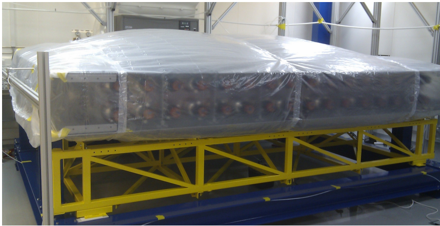
Figure 13.5.: Photograph of the anti-radon tent covering the C-section.
