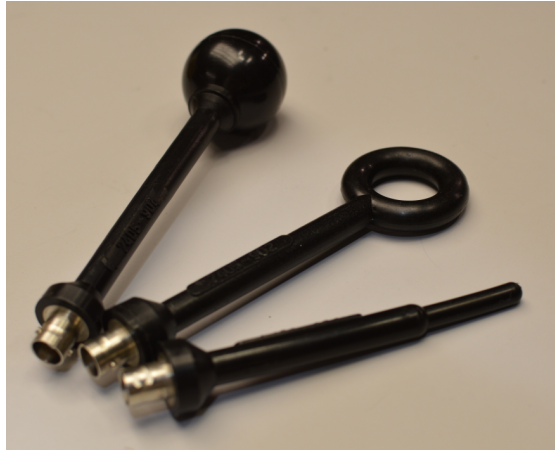
Figure 8.3: The E and H near-field probes, manufactured by ETS-Lindgren. The magnetic field probe is in the middle and the two probes on the side are electric field probes (The left ball probe generates a wider field than the right stub probe).
