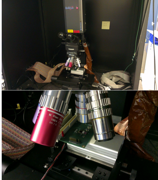
Figure 6.9: The laser set-up showing the laser head and the DAQ board. The laser system has a built-in microscope camera which helps guide the laser through the strips.
