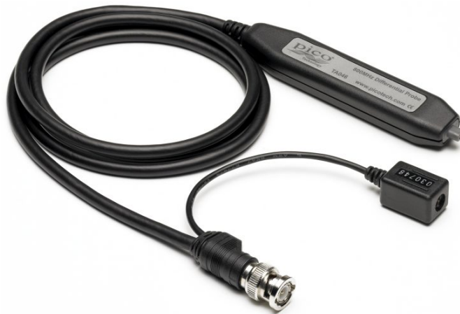
Figure 6.16: The Pico TA046: 800 MHz, 15 V active differential oscilloscope probe used in the measurements.
