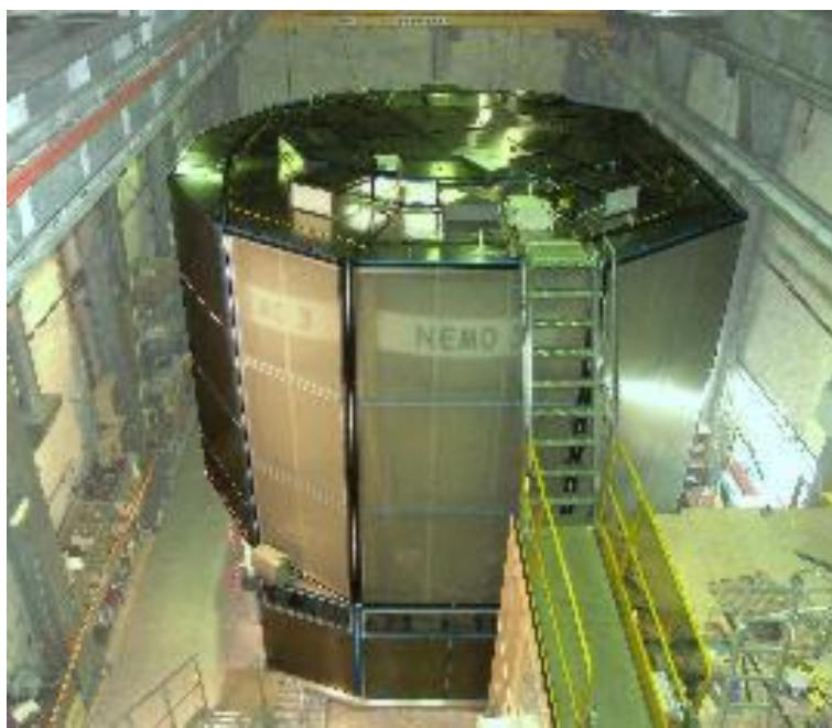
Figure 5.5: Photograph of the radon tent surrounding NEMO 3 after installation.
