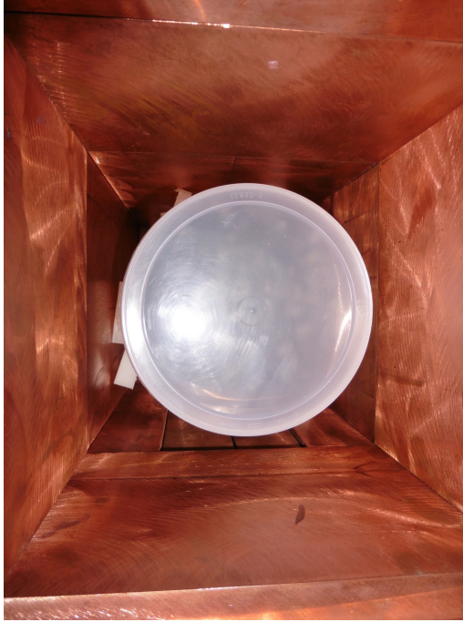
(a) Sample on HPGe detector for measurement.
