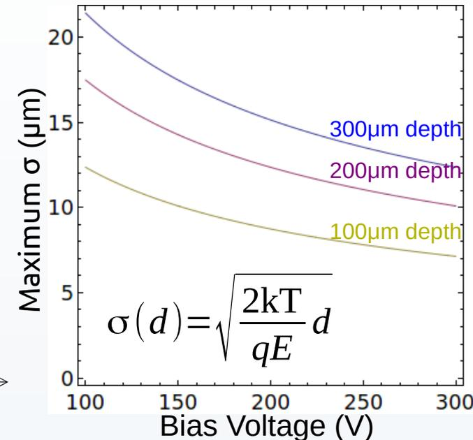
The width of this spread depends on interaction depth and the electric field due to the bias voltage
