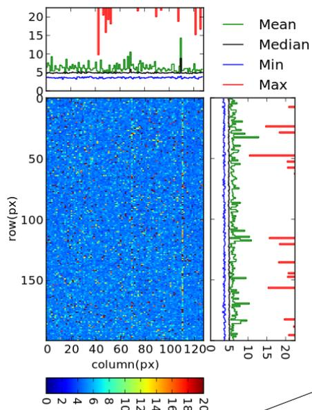
Noise map and histograms from simulated (Left) and measured (Right) dark frames
