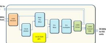
The clocking circuitry includes a local crystal oscillator, PLL and non-PLL based multiplexers in order to provide an uninterrupted, stable clock to the final PLL which multiplies the bunch clock to provide the 99 MHz clock. This clock then goes into a 1:16 LVDS fanout chip. A copy of this clock also goes back to the DAMC2/FPGA through the RTM connector.
