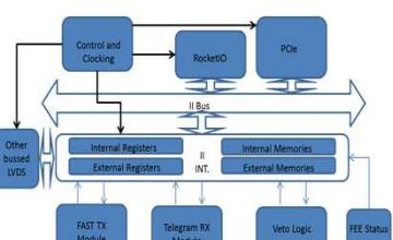
The FPGA firmware for the CC system is built around a bus/register structure called the II Bus, whose registers are accessed through either the PCIe link to the crate processor or the blocks attached to the bus. The EuXFEL central software system controls the CC system through the PCIe link.
