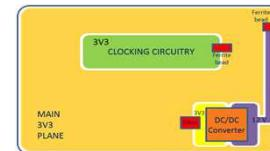
We envisage further improvements when this filtering scheme is employed on the final version of the CC RTM and the voltage plane for the clocking circuitry is separated from the main power plane by a ferrite bead.
