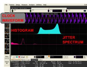
The current configuration of the CC RTM showed a high TIE and period jitter reading on the 99 MHz clock with the shape of the histogram suggesting a high amount of deterministic jitter. The high peak around the 780 KHz and a smaller peak at double this frequency in the jitter spectrum corresponds to the switching frequency of the DC/DC converter, LTM4600EV. Therefore, the main jitter contribution comes from the ripple on the 3.3 V output from the DC/DC converter.
