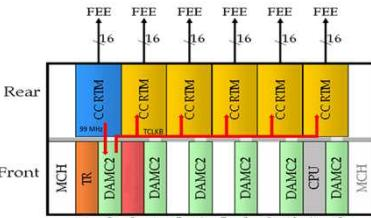
In order to synchronise the operation of the master and the slave boards, 99 MHz clock generated on the RTM is put on the TCLK1 line on the MTCA.4 backplane. The new version of DAMC2 board currently developed by DESY supports this feature. With the slave boards in the same 12-slot crate up to a 6 mega pixel detector can be supported.
