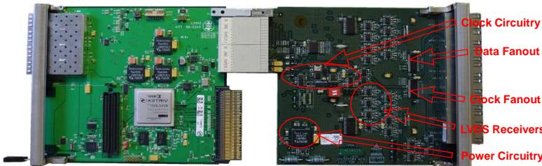
The CC system is responsible for the synchronisation of the detectors and the DAQ system to the general EuXFEL timing. The EuXFEL facility will generate coherent and intense X-ray flashes with a ~4.5 MHz bunch frequency. The Timing Receiver (TR) board housed in the same crate as the CC system delivers the bunch clock to the CC through the MTCA.4 backplane.
