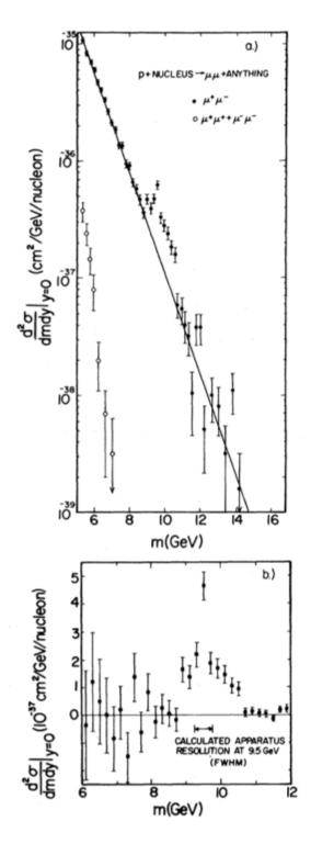
Figure 12: Distribution of Invariant mass of pairs of muons, showing clear enhancement above the continuum at about  $9.5\,\mathrm{GeV}$ . From [16].
