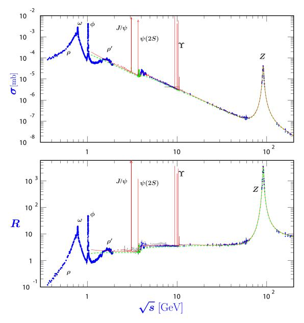
Figure 7: Measurement of the total cross section,  $e^+e^- \to \text{hadrons}$ , and ratio,  $e^+e^- \to \text{hadrons}/e^+e^- \to \mu^+\mu^-$ , as a function of the centre-of-mass energy,  $\sqrt{s}$ . The curves are a guide using simple theoretical models. From [14].
