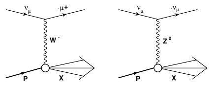
Figure 2: Feynman cartoons of the (left) charge current and (right) neutral current processes for neutrino-proton collisions.
