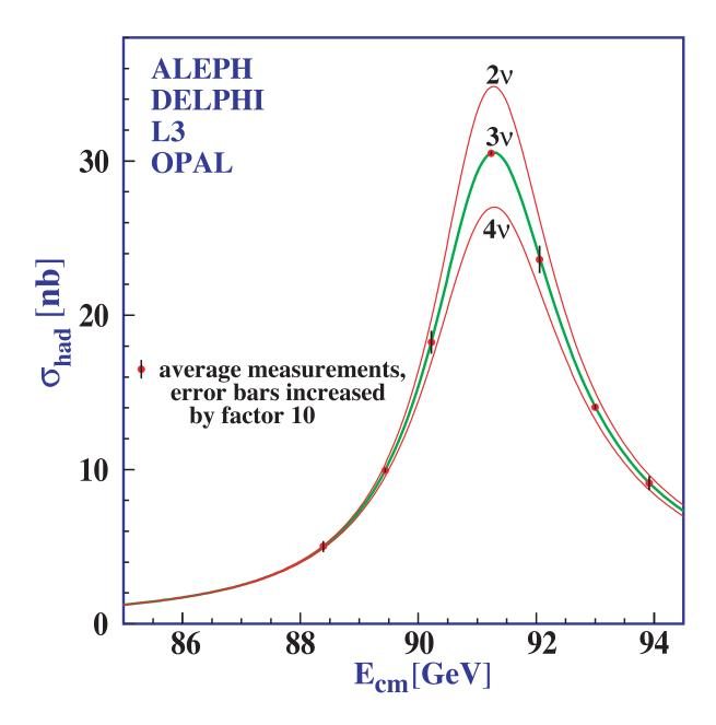
Figure 9: Combined LEP data on the cross section,  $e^+e^- \to \text{hadrons}$ , as a function of centre-ofmass energy near  $M_Z$ . The curves show the predictions of the Standard Model with two, three, and four species of light neutrinos. The asymmetry of the curve is produced by initial-state radiation. Note that the error bars have been increased by a factor ten for display purposes. From [14, 15].
