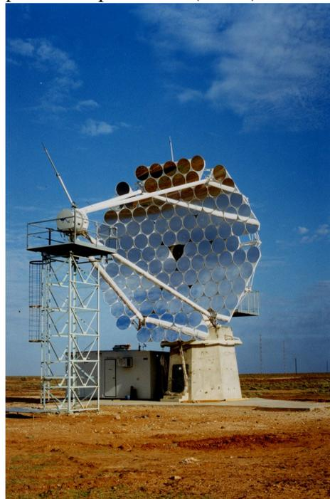
**Fig.22: The CANGAROO-II (Collaboration of Australia and Nippon for a GAMMA Ray Observatory in the Outback)** is a project based near Woomera in South Australia, which was set up to study sources in the southern sky that emit  $\gamma$ -rays in the TeV range. The 10m reflecting ACT is shown during the day in its stowed position ([www.icrhp9.icrr.u-tokyo.ac.jp](http://www.icrhp9.icrr.u-tokyo.ac.jp))
