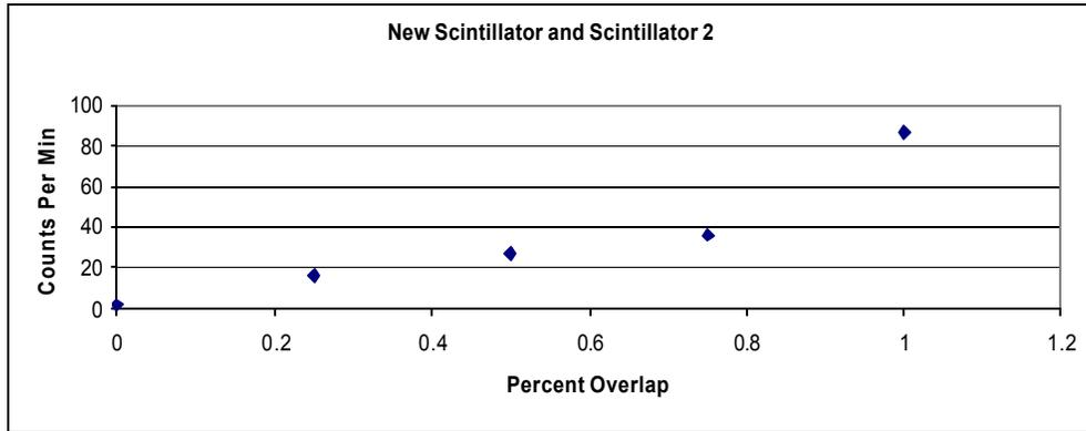
Fig. 51: Graph showing the 2-way coincidence results for the new scintillator and scintillator 2
