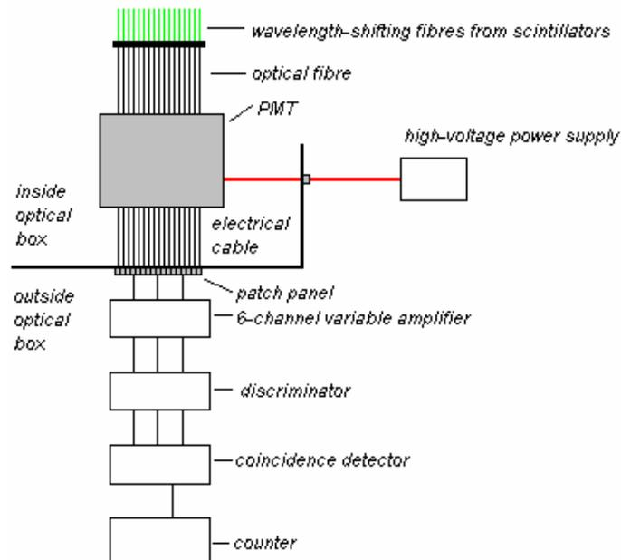
**Fig.29: Schematic diagram of the optical and electrical components of the test stand**
