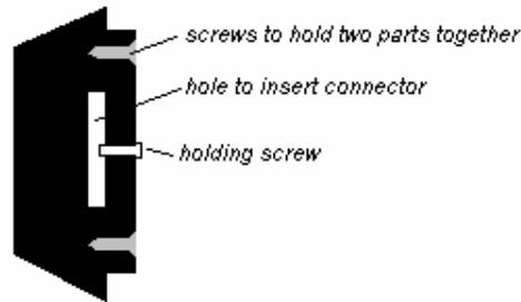
**Fig.66: Jig used to polish the wavelength-shifting fibres**
