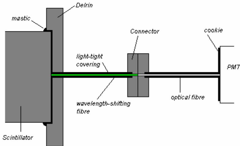
**Fig.67: Schematic diagram of the optical connections.** This is shown for a single fibre but in the detector the fibres were connected in pairs to reduce the number of connectors required.
