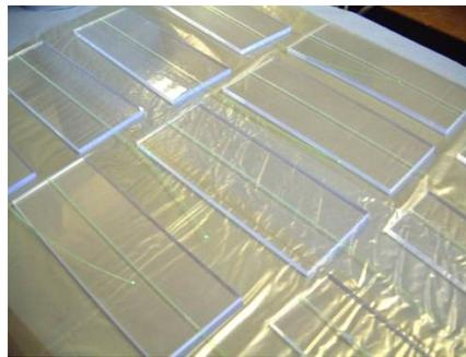
**Fig.63: Scintillators after the gluing process**
