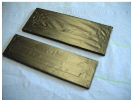
**Fig.64: Two of the wrapped scintillators**
