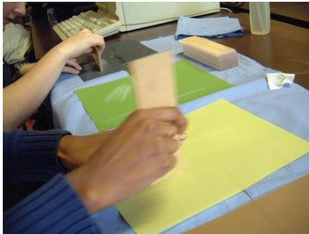
Fig.62: Polishing the scintillators
