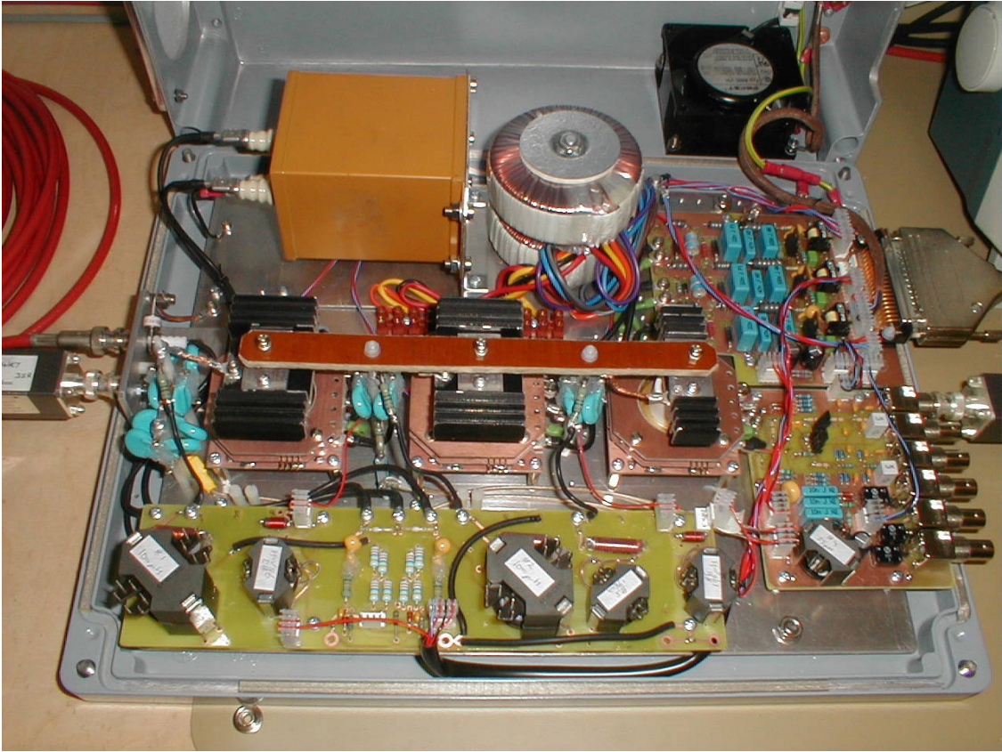
Figure 5.31: The electronics layout within the FONT kicker amplifier. The three planar triodes are encased within the black heat sinks in the centre of the box. The feedback signal and trigger inputs are on the right hand end of the box, with the high voltage supply input and kicker supply output on the left.
