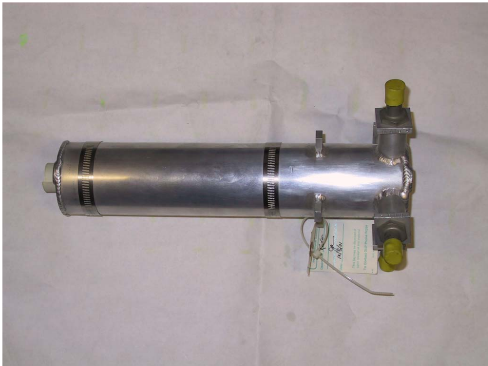
Figure 5.16: The SLC Scavenger Post Kicker magnet used in the construction of the FONT integrated magnet assembly. The input connectors are covered by yellow protective caps, on the right hand end of the kicker barrel.
