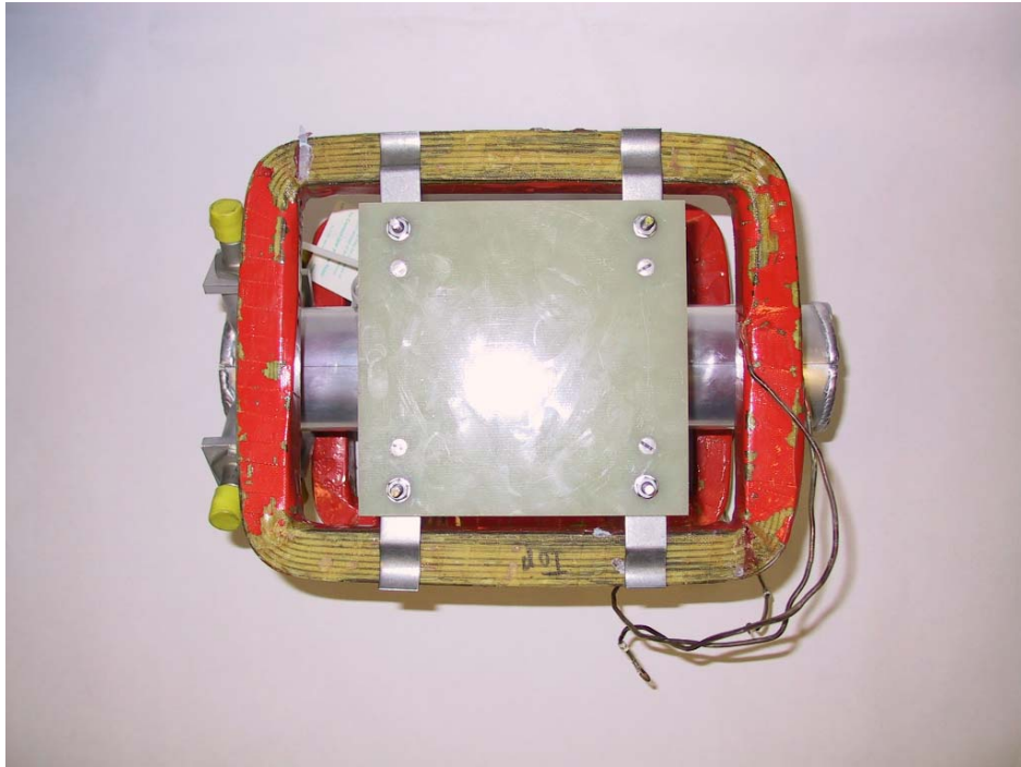
Figure 5.5: The FONT integrated magnet assembly. The dipole coils are red and mounted around the silver barrel of the kicker magnet.
