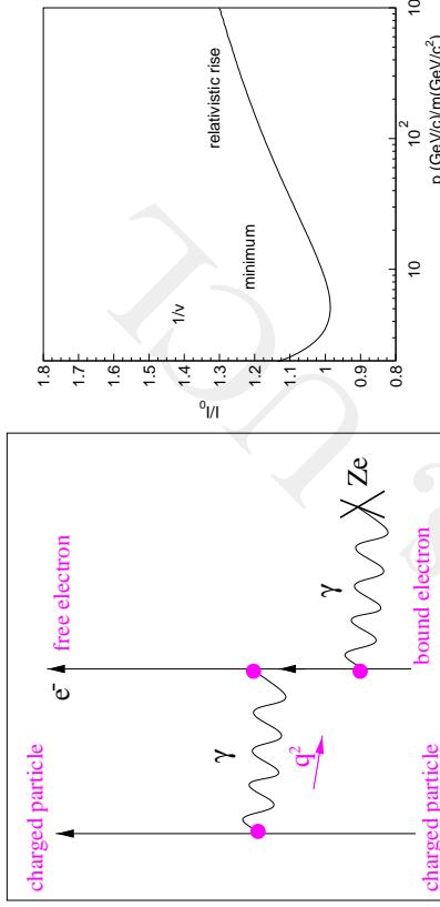
Figure 39: Left:Feynman Diagram for Ionization energy loss for a charged particle. Right: Shape of the Bethe-Bloch energy loss function
