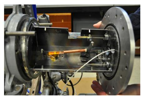
Simple proto-oven made of copper with a tungsten wire heater + ceramic insulators
