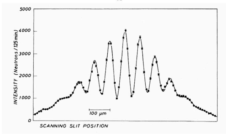
BF<sub>3</sub> detectors were used to scan across horizontally and the number of neutrons were counted at regular intervals.
