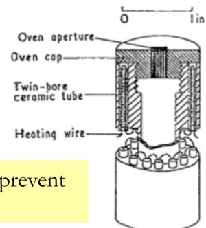
Heat the aperture and collimator to prevent build up of atoms of aluminium.
