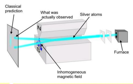
The observation is a beam split into two parts: spin-up, spin-down.
