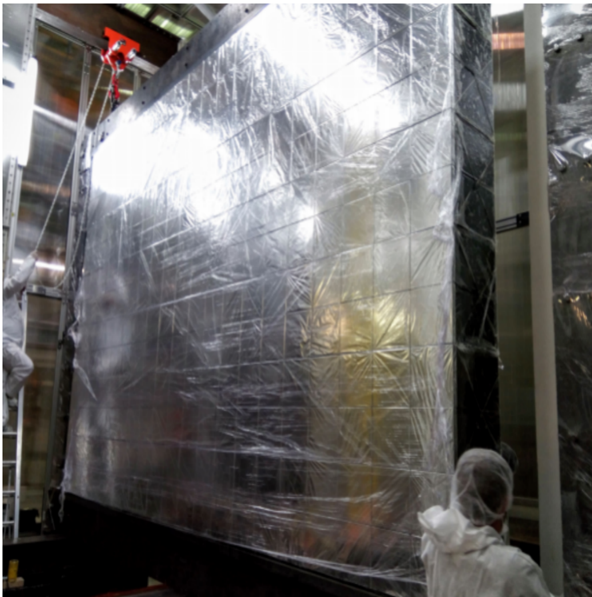
Figure 3.5: One of the Main Walls assembled at the LSM. Each Main Wall contains 220 8" calorimeters and 40 5" calorimeters [56].
