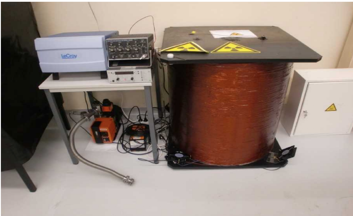
Figure 3.17: Image of the copper solenoid and impermeable container used to measure the ability of the shields to remove the magnetic field within their volume [118].
