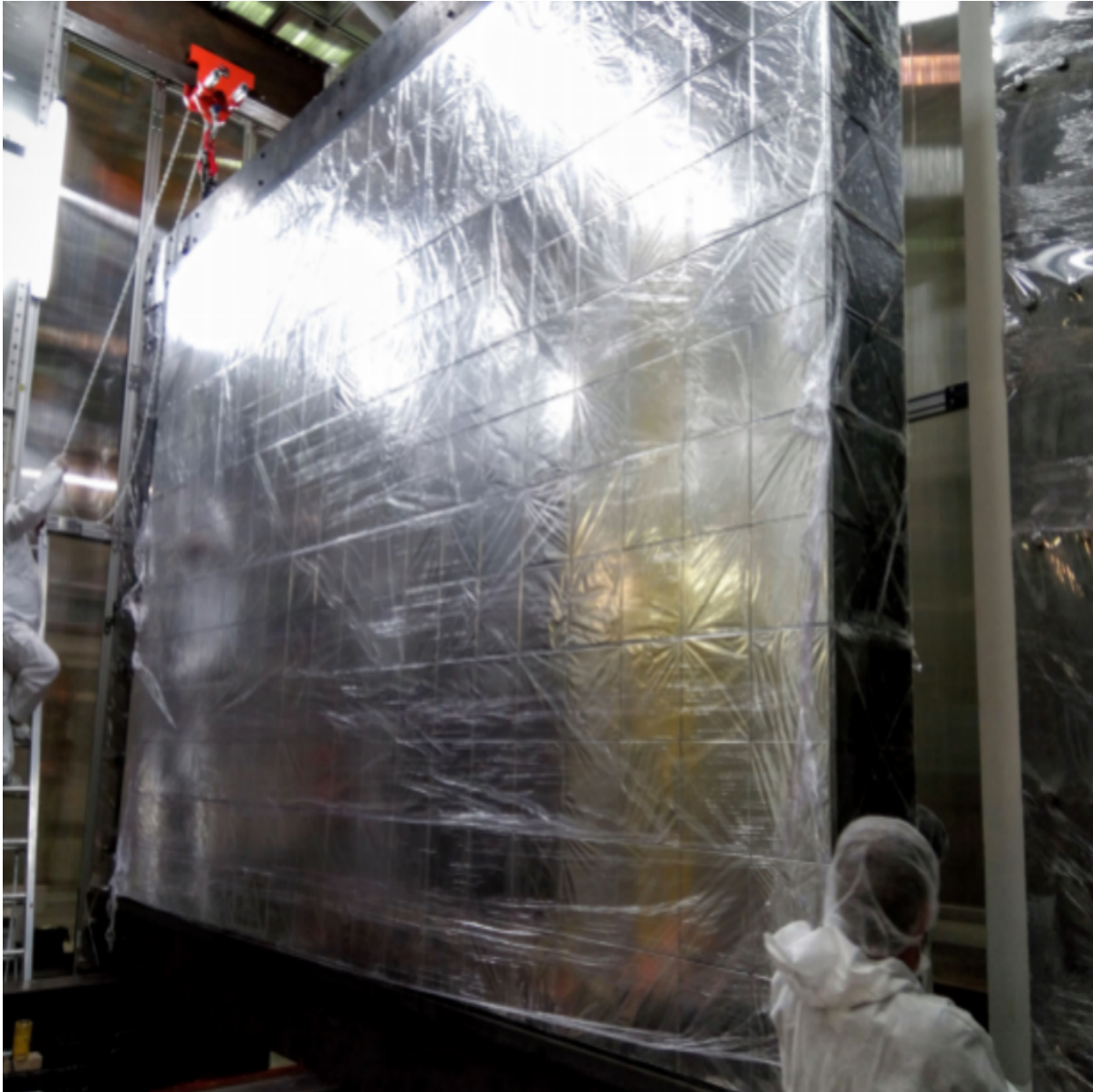
Figure 3.5: One of the Main Walls assembled at the LSM. Each Main Wall contains 220 8" calorimeters and 40 5" calorimeters [50].
