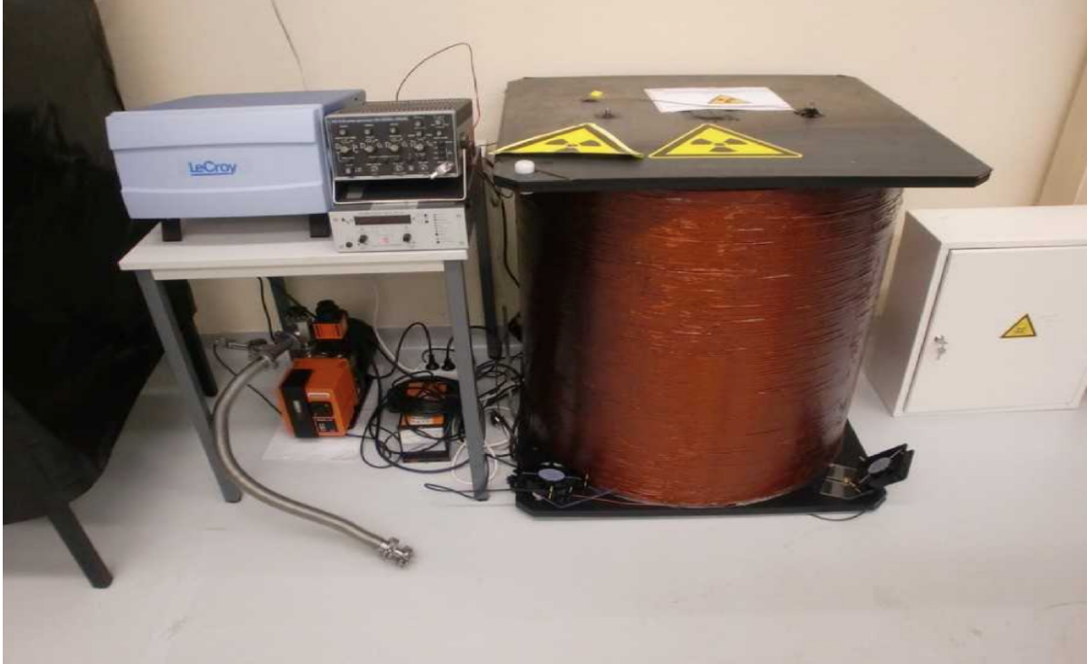
Figure 3.18: Image of the copper solenoid and impermeable container used to measure the ability of the shields to remove the magnetic field within their volume [111].
