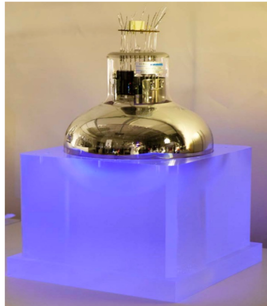
(b) SuperNEMO optical module, including a PMT coupled to the plastic scintillator in Figure 3.3a.
