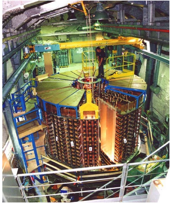
Fig. 2. View of the NEMO 3 detector in the LSM before the installation of the last sector.
