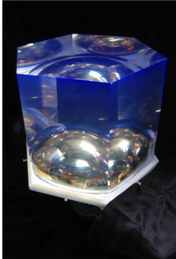
Figure 1: A PVT scintillator block directly coupled to a high-QE 8" PMT. The block is 19.3 cm deep and the minimum thickness of scintillator between the front face and the PMT mounted at the rear is 10 cm. This device was found to have the best resolution for MeV energy electrons.
