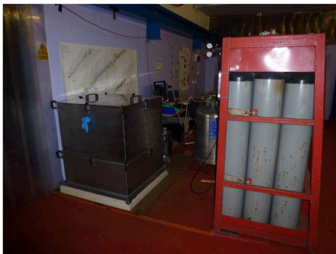
Figure 22: The radon tent fully constructed and clamped down around the detector with the cylindered nitrogen rack on the right.
