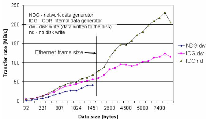
Fig. 4. ODR through-put performance. All measurements with a single requester thread, single IO thread (disk write). Data is written to a disc-array, with Events stored in groups of 10000 events written to the same file.
