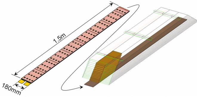
Fig. 2. ECAL slab shown in the context of the EUDET module-0 design.
