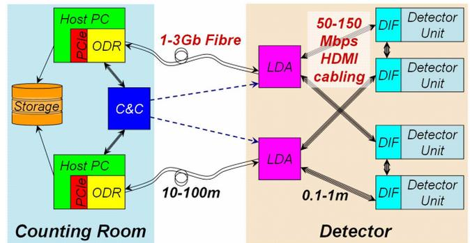
Fig. 3. CALICE DAQ structure, showing the various modules of the system.
