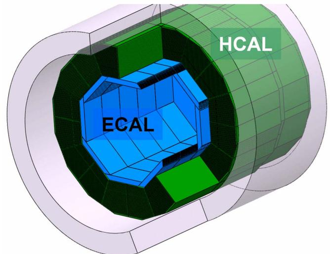
Fig. 1. The geometry of a calorimeter inside an ILC detector
