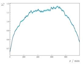
The amount of light collected from the screen varies with position due to the finite optics size. This was measured by scanning a known light source across the screen and measuring the relative brightness.
