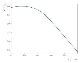
Electrons are incident on the plane of the screen at different angles  $(\theta_j) \Rightarrow$  different path lengths within the scintillator. Scintillator response  $\propto$  path length, so correction must be applied.
