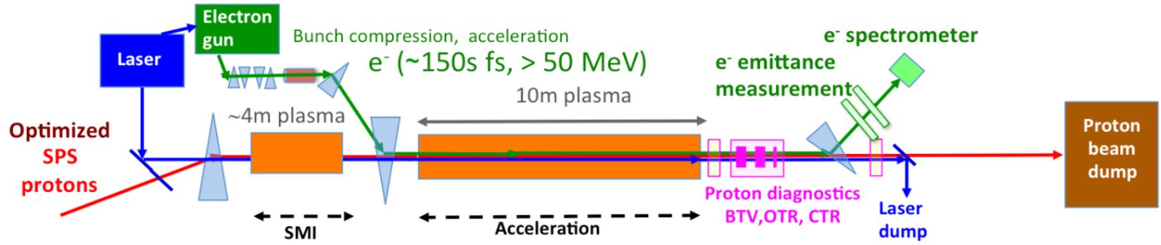
Preliminary Run 2 electron beam parameters
