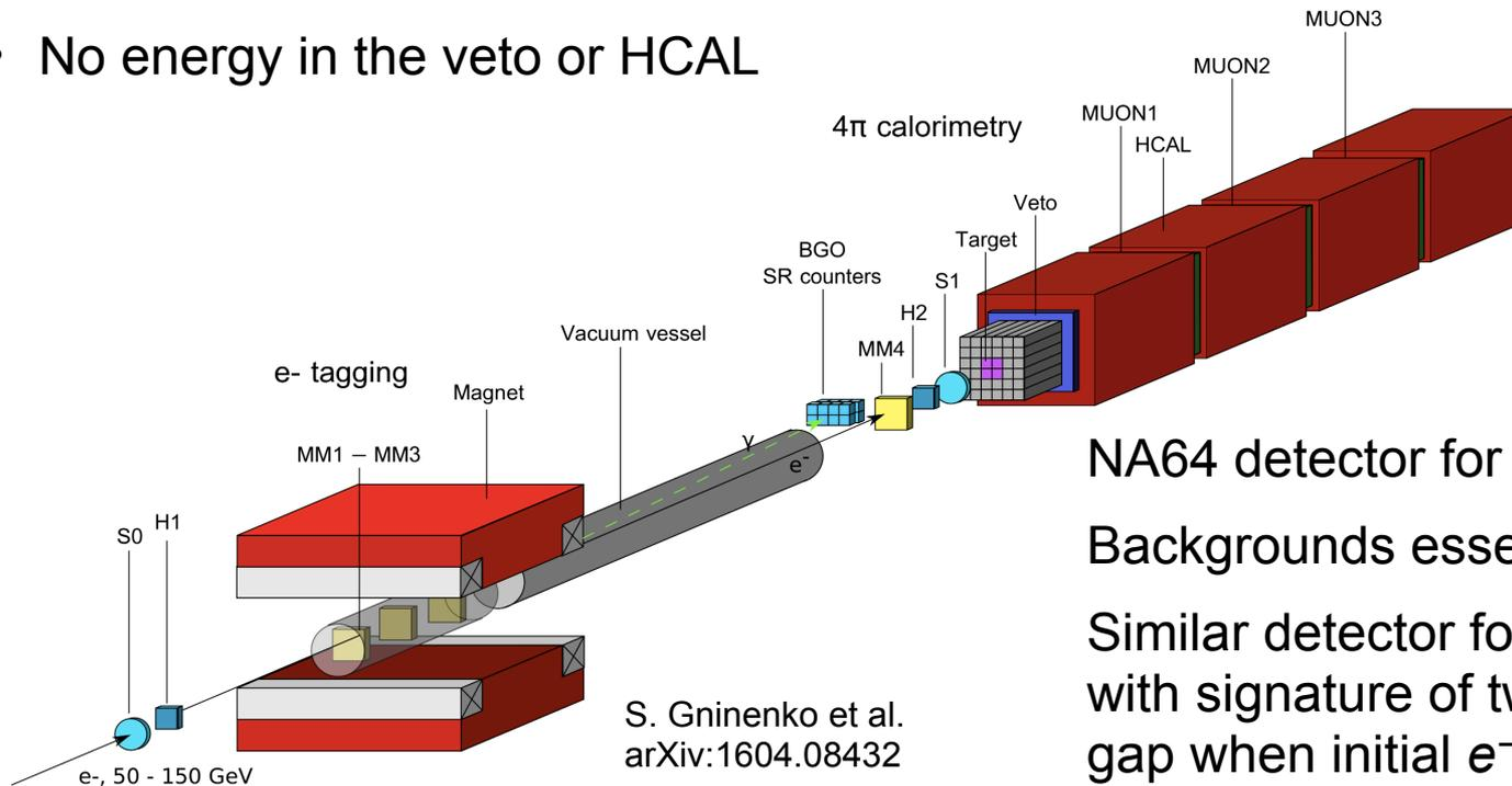
NA64 detector for  $A' \rightarrow \textit{invisible}$  channel.
