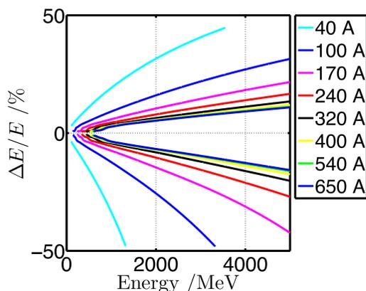
Figure 3.  $\Delta E/E$  vs. energy for dipole HB4 at various current settings.
