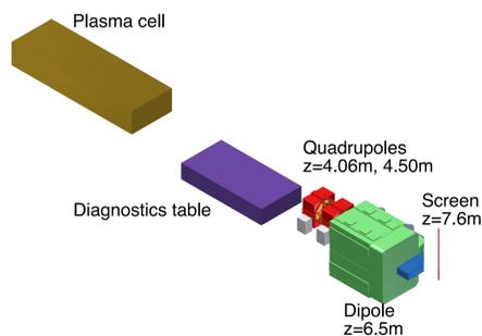
Figure 1. Layout of the spectrometer system.
