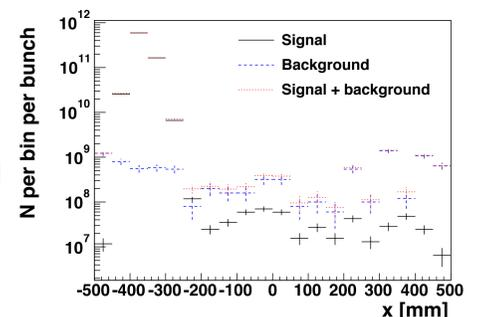
Figure 6. Optical photons emitted from the screen due to signal (witness electrons) and background in the screen.
