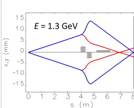
Figure 4. ELEGANT simulation results showing the trajectories of electrons with initial angles of  $\pm 2$  mrad. The quadrupoles have  $K_1 = \pm 4.07 \text{ m}^{-2}$
