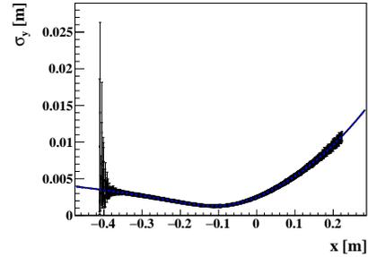
Fig. 2. A fit of the beam size function to the simulated spectrometer output. The black line is the input function. The dashed blue line is the fit (the lines are almost entirely overlapping)
