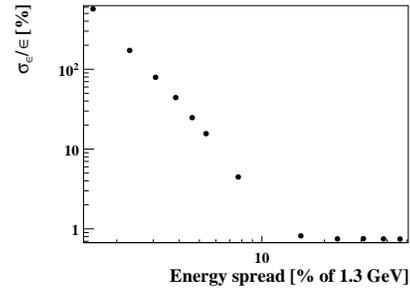
Fig. 3. Calculated uncertainty of the simulated emittance measurement vs. energy spread.
