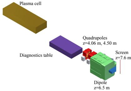
Fig. 1. A 3D CAD image of the spectrometer system annotated with distances along the  $z$  direction from the exit of the plasma cell to the magnetic centers of magnets, and the center of the scintillator screen.
