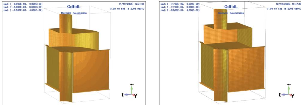
**Figure 1:** Baseline cylindrical (left) and alternative rectangular ( right) shapes of the cavity BPM
