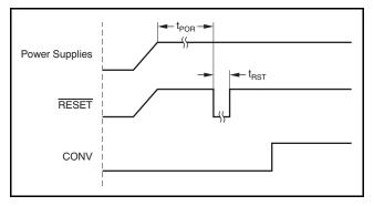
Figure 24. DDC232 Timing at Power-Up
