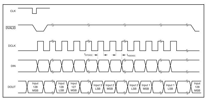
Figure 19. Timing When Using DDC232 DIN Function; See Figure 18
