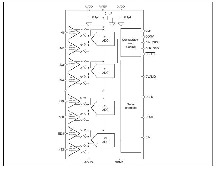
Figure 2. DDC232 Block Diagram
