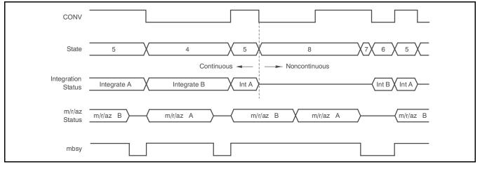
Figure 15. Changing from Continuous Mode to Noncontinuous Mode
