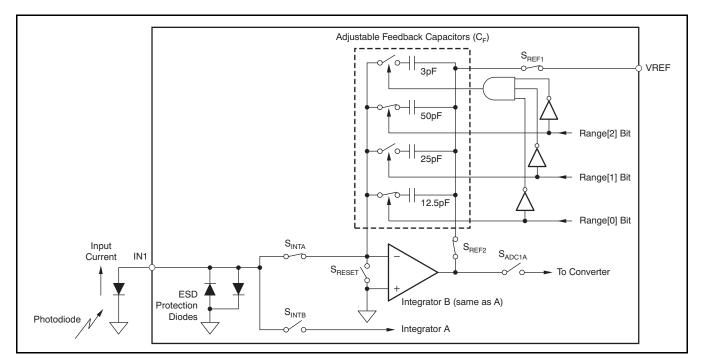
Figure 3. Basic Integration Configuration for Input 1
