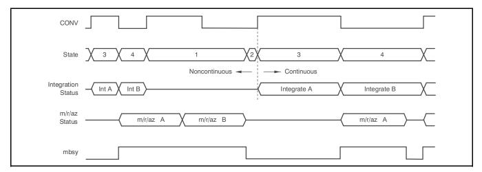
Figure 16. Changing from Noncontinuous Mode to Continuous Mode
