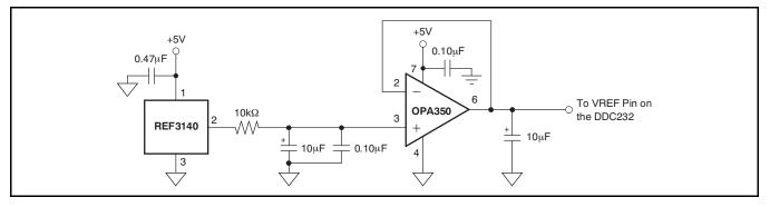
Figure 6. Recommended External Voltage Reference Circuit for Best Low-Noise Operation
