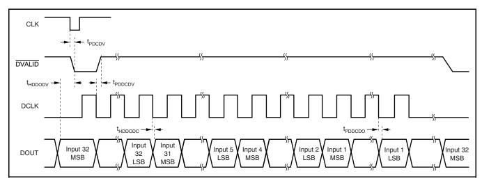
Figure 17. Digital Interface Timing for Data Retrieval From a Single DDC232
