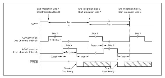
Figure 12. Internal Operation in Continuous Mode Timing
