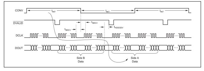
Figure 22. Readback *Before* and *After* CONV Toggles
