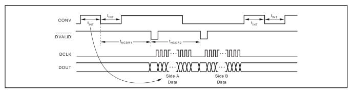
Figure 23. Readback in Noncontinuous Mode
