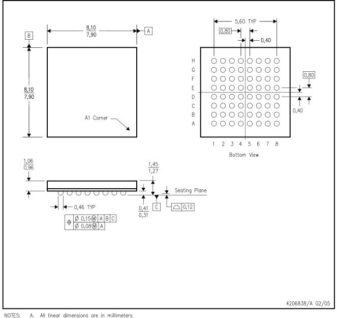
Α. All linear dimensions are in millimeters.
