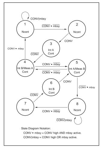
Figure 10. Integrate/Measure State Diagram
