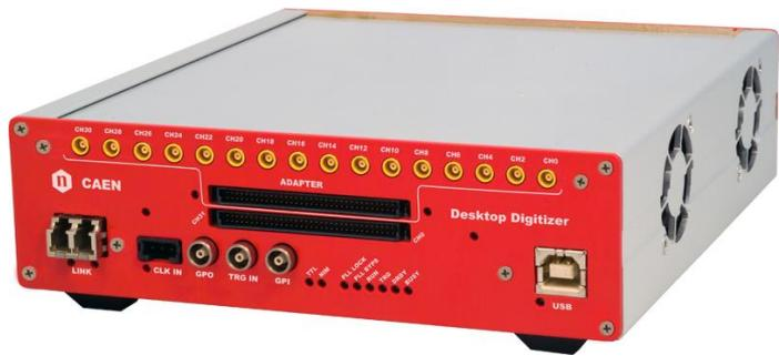
16 channels are also available on MCX coaxial connectors, while the A746E Adapter is required for all the 32 channels to be available on as many single-ended LEMO connectors (see § 2.5.1). Because of the high channel density, provided by the AD9222 Octal 12-bit 65 MSPS Analog-to-Digital Converter, most channel settings are performed over “groups” of 8 channels (one group per ADC chip).
