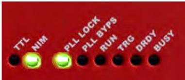
Fig. 11.1: Front panel LEDs status at power-on.
