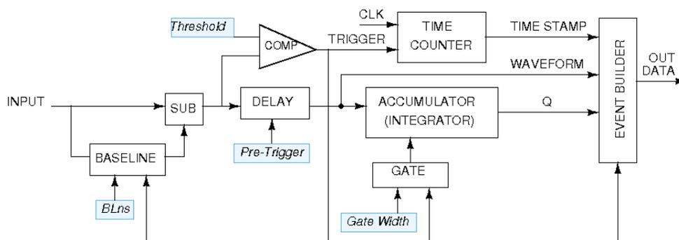
**Fig. 2.1:** Functional Block Diagram of the DPP-QDC
