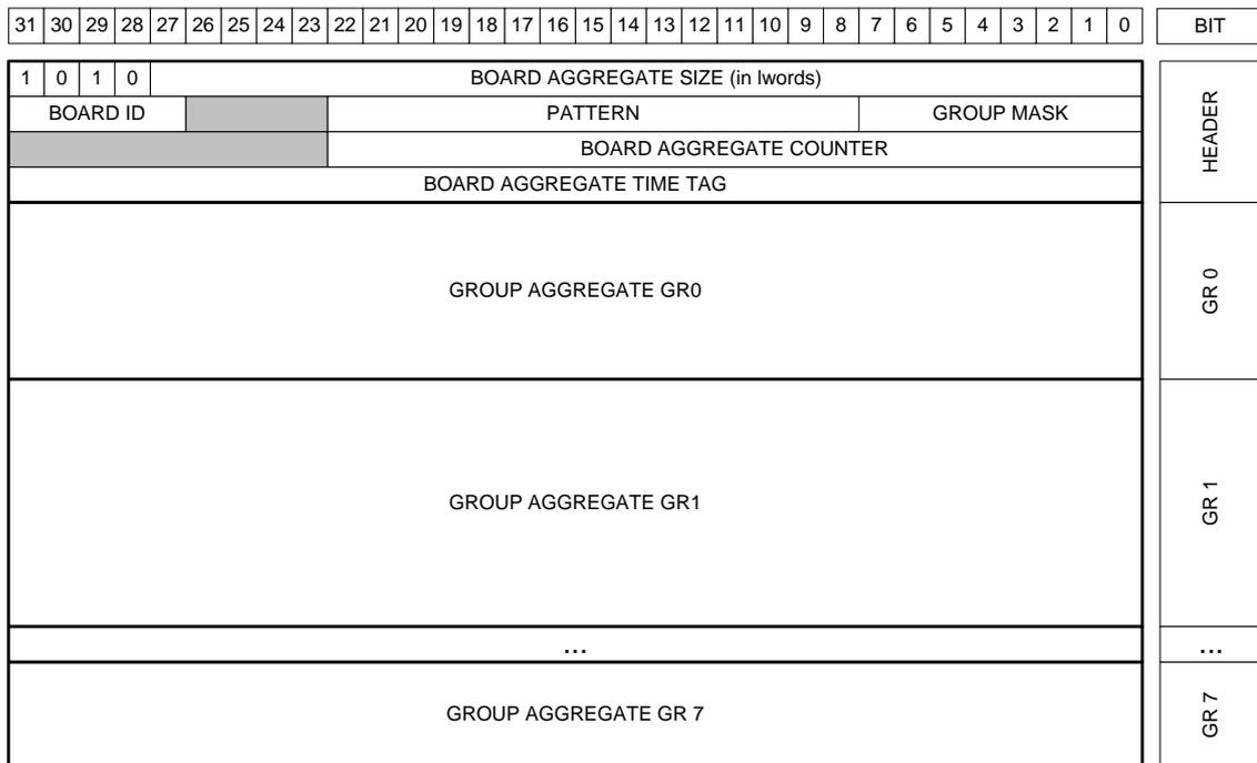
Fig. 4.2: Board Aggregate Data Format scheme for 740D series
