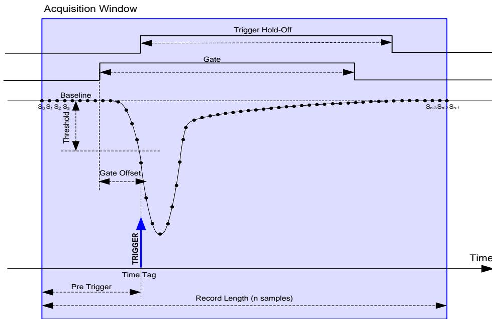
**Fig. 2.2:** Diagram summarizing the DPP-QDC parameters. The trigger fires as soon as the signal crosses the threshold value. Gate, Gate Offset, Pre-Trigger, Trigger Hold-Off, and Record Length are also shown for one acquisition window
