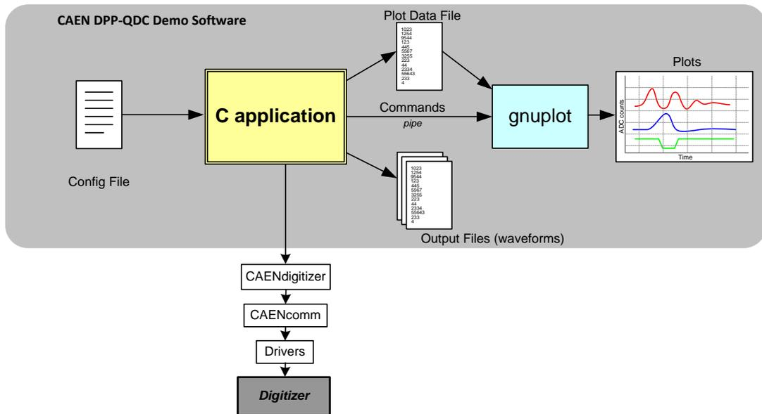
**Fig. 5.1:** The DPP-QDC Demo Software block diagram
