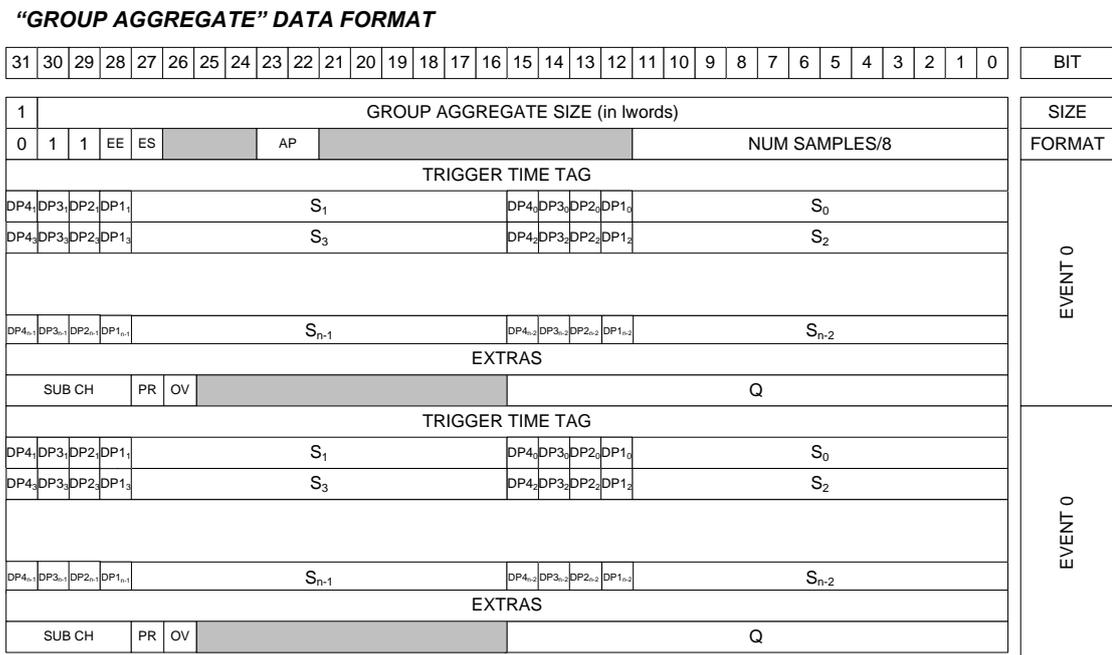
Fig. 4.1: Group Aggregate Data Format scheme for 740D series
