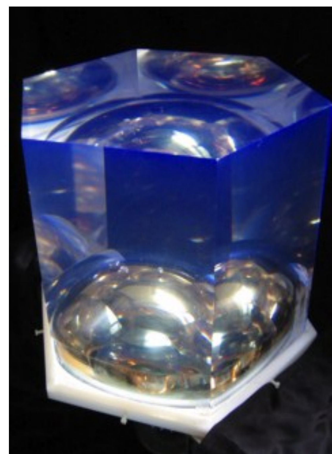
Figure 1: A PVT scintillator block. The block is 19.3 cm deep and the minimum thickness of scintillator between the front face and the PMT mounted at the rear is 10 cm. This device was found to have the best resolution for MeV energy electrons.
