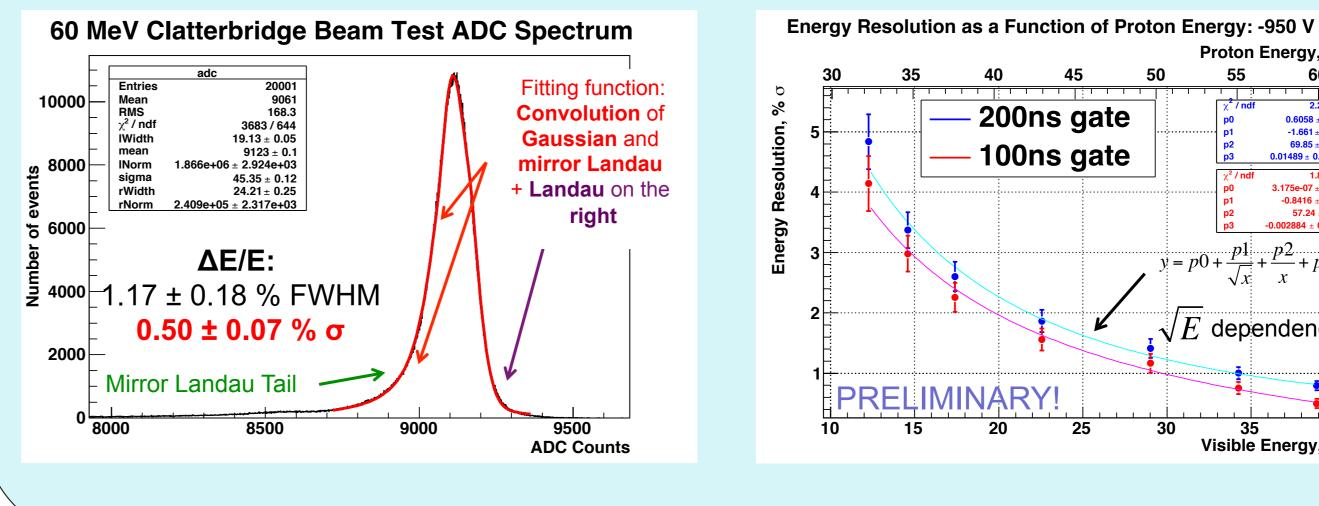
decrease beam energy and measure  $\Delta E/E$  as a function of proton energy:
