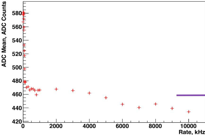
Hamamatsu Base PMT at -900 V Pulsed with LED: 1 mA Peak Current, ET, Long Scintillator
