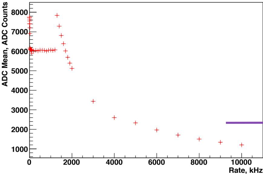
Hamamatsu Base PMT at -1200 V Pulsed with LED: 12 mA Peak Current, ET, Long Scintillator
