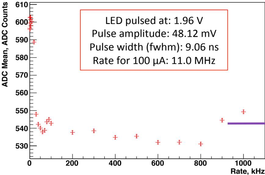
Hamamatsu Base PMT Pulsed with LED: 1 mA Peak Current, ET
