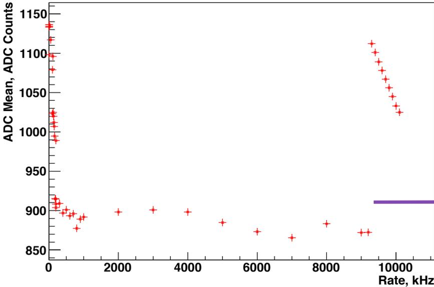
Hamamatsu Base PMT at -1200 V Pulsed with LED: 2 mA Peak Current, ET, Long Scintillator
