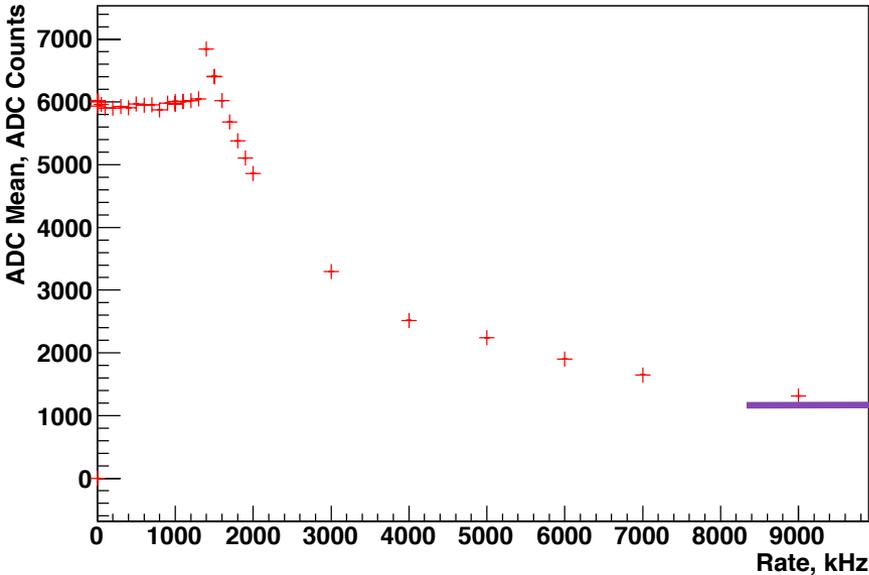
Hamamatsu Base PMT at -1200 V Pulsed with LED: 12 mA Peak Current, ET
