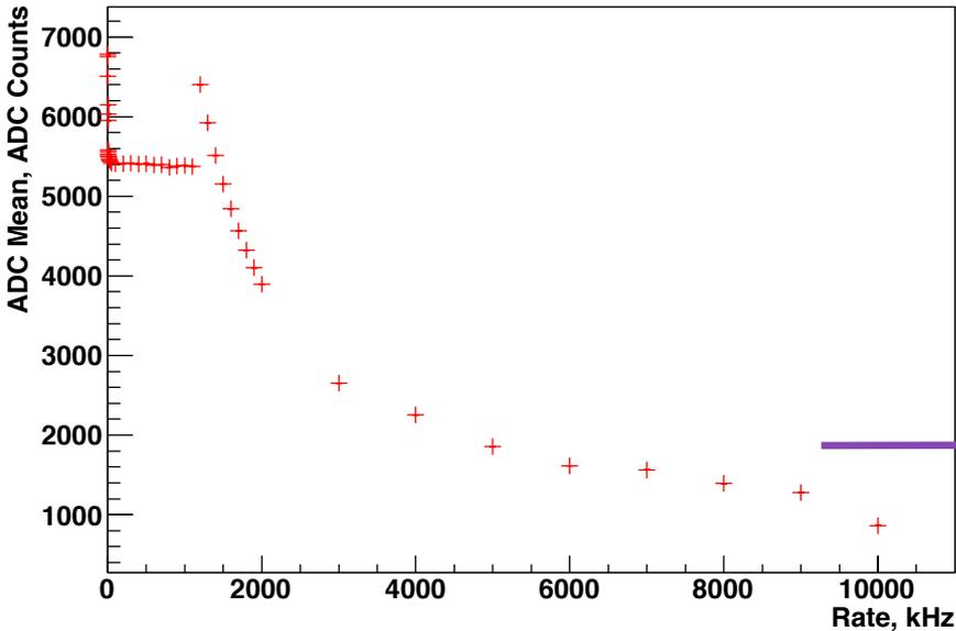
Hamamatsu Base PMT at -900 V Pulsed with LED: 10 mA Peak Current, ET, Long Scintillator
