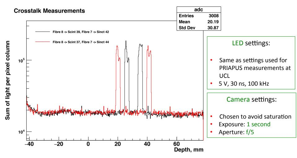
Conclusion: just as with single fibre tests we do not see any crosstalk!
