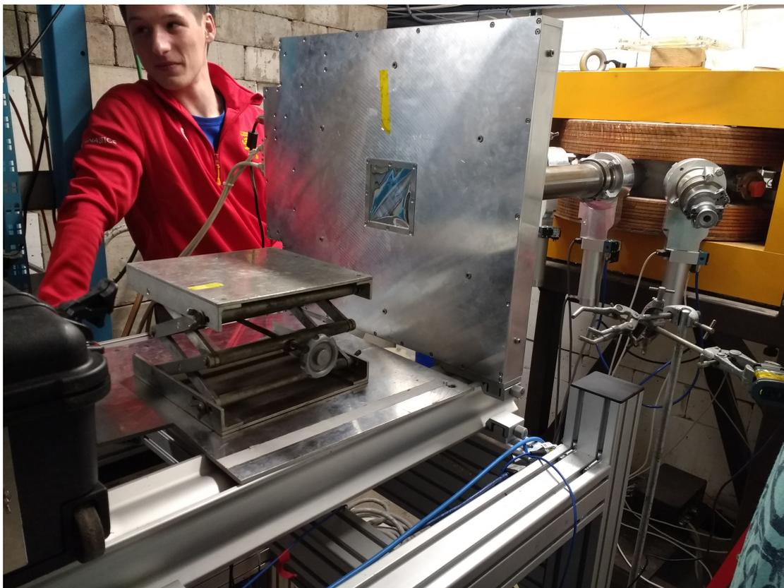
**Figure 12:** The PRaVDA tracker module mounted on the bench in front of the beam nozzle. The stand on which the UCL calorimeter prototype was placed can be seen in front of the tracker.
