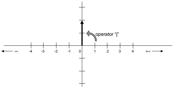
This multiplies the number 2 by an *operator* that rotates it anti-clockwise by a right angle. If we do this operation twice,  $j(j(2)) = j^2.2$ :
