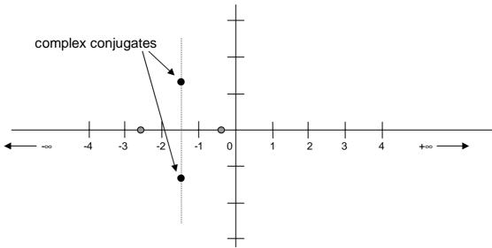
The grey dots show the first pair of roots (both real) and the black dots the second pair (both complex). Notice that the complex pair are mirror images of each other. This always happens when roots are found. Complex numbers like this with equal real parts and opposite imaginary parts are called *conjugate*.
