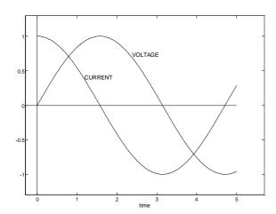
$i = \omega C v_p \cos(\omega t)$ . This shows that the current has an amplitude that is proportional to the voltage (Ohm's Law) but that the current leads the voltage by 90°.
