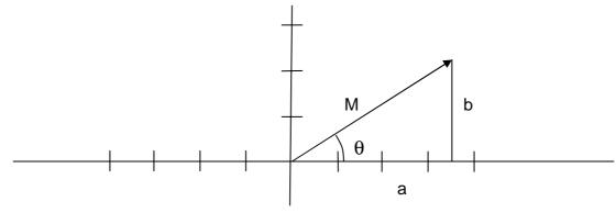
The number is represented by a magnitude M and a phase  $\theta$  where  $a=M.\cos(\theta)$ ,  $b=M.\sin(\theta)$ ,  $M=\sqrt{(a^2+b^2)}$ ,  $\theta=\tan^{-1}(b/a)$ .
