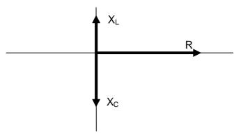
We can now represent the effect of more than one component, just as we can for several resistors, but when there are capacitors and/or inductors present too. The relationship between the voltage and current is now, generally, neither *in-phase* (purely resistive) or *in quadrature* (purely reactive), and is called the **impedance**.
