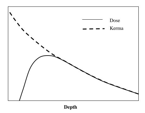
• kerma is highest at entry point and then decreases due to photon attenuation In order to relate absorbed dose to kerma and exposure mathematically we need to introduce the concept of charged particle equilibrium CPE.
