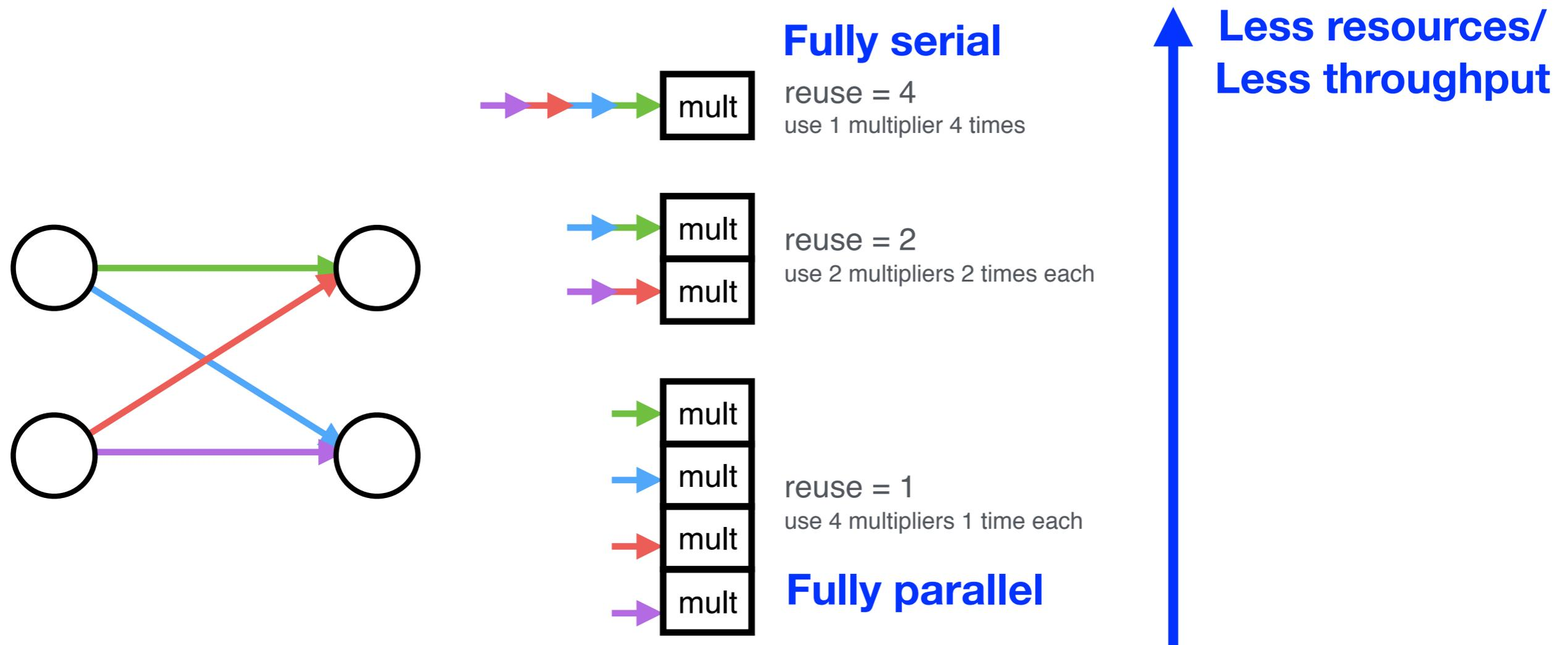
**Reuse factor:** how much to parallelize operations in a hidden layer
